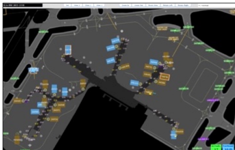
Display/Interface Ramp Traffic Console (RTC): Flight info, pushback advisories
